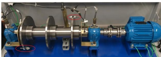
Fig. 3 laboratory test bench for unbalance fault [14]
