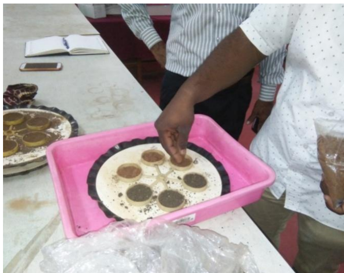
Fig. 2- Field capacity determination by pressure plate apparatus
