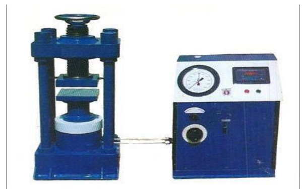
Fig.5.2.5 Compression Testing Machine
