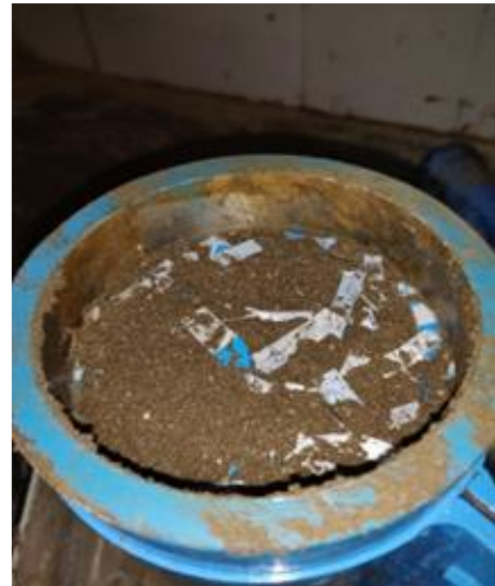
Figure 3 - CBR sample of PW reinforced marine clay
