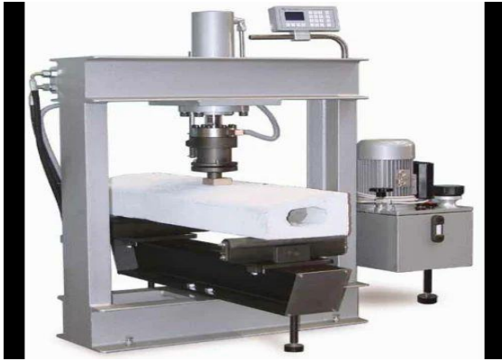
Fig.5.2.6 Flexural Strength Testing Machine
