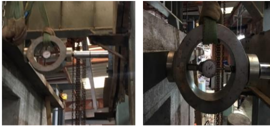
Fig.4 Loading arrangement with hydraulic jack
