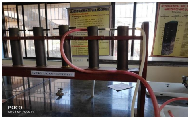
Fig. 3 - Experimental setup for Hydraulic Conductivity by constant head method
