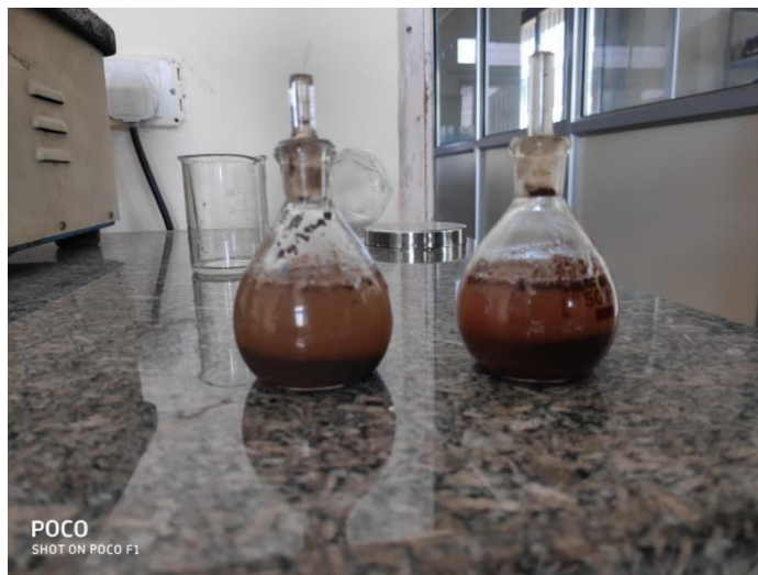
Fig.5 - Particle density experimentation (by pycnometer method)
