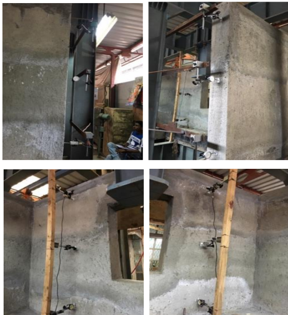
Fig.5 Arrangement of potentiometer and dial gauge
