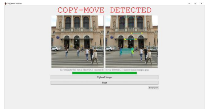
Fig 10. Forgery Detected in Image using SIFT Algorithm
