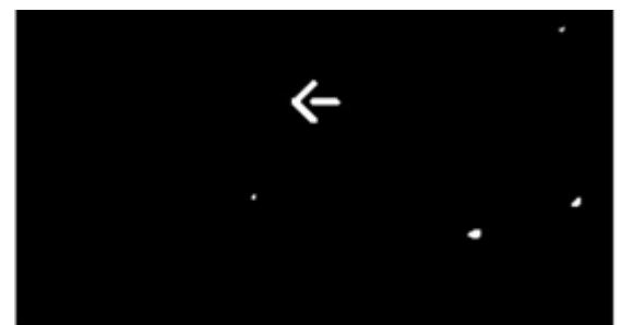
Fig. 6.2 Applying colour thresholding to the processed image
