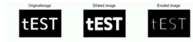
Fig. 5.4 Left the original image. Center the dilated object. Right the eroded object. Graphic by OpenCV
