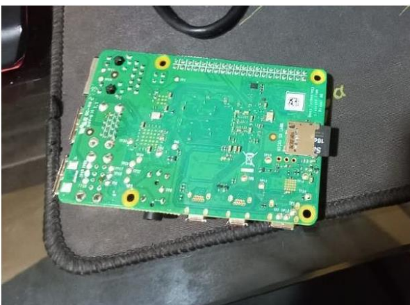
Fig. 7. SD card inserted in RPi 4
