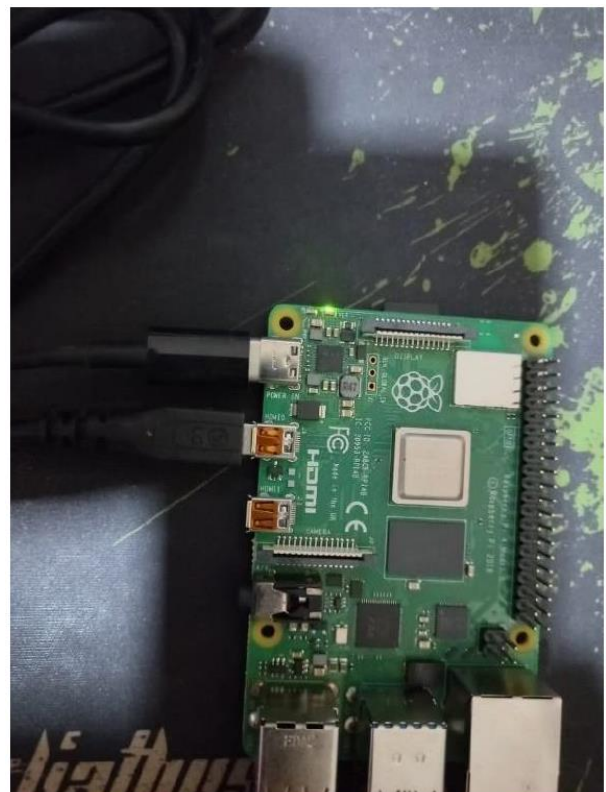
Fig. 9. Connecting power supply to the ARM SBC (RPi 4)
