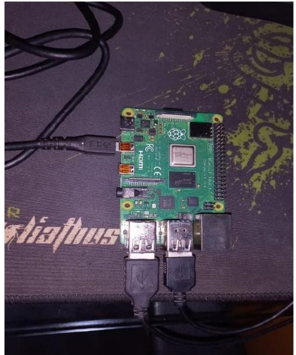
Fig. 8. Peripherals connected to the ARM SBC (RPi 4)
