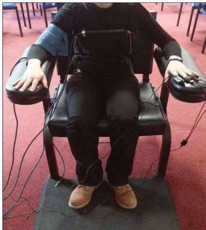
Figure 3. Polygraph equipment attached to an examinee
